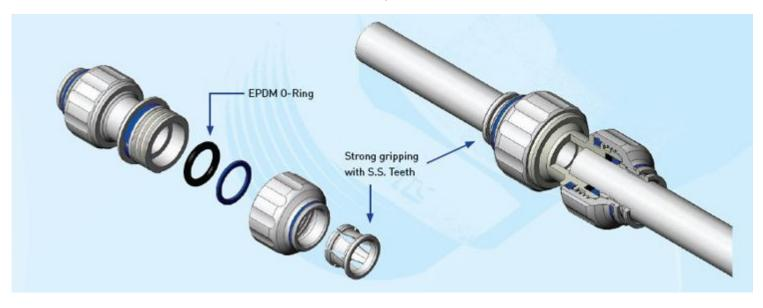
• Ensure that the tubing is pushed into the fitting fully past both the collets [gripper] and the 'O' ring and is engaged properly in accordance with the manufacturer's instructions.
