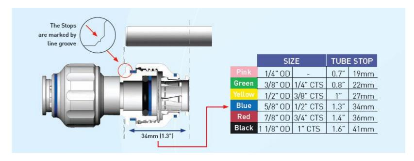
**Twistloc®** fittings should be in the "unlocked" position, this shown by coloured line which a small gap between the screw cap and the body. Ensure that they are kept free from scratches, gouges, dirt and debris or any form of damage on the circumference of all fittings.
