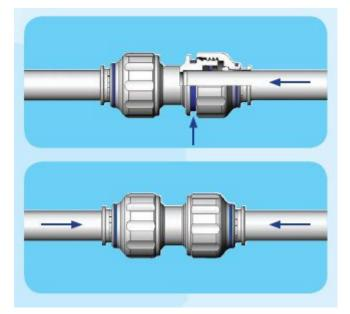
Ensure no scratches, gouges or any form of damage on the circumference of the tubing within one [1] inch [24.4mm] of the cut end. Damage in this area may cause leakage problem.
